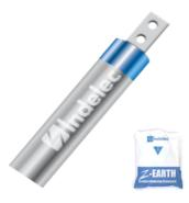
Hot Dip Galvanized with 80-100 micron, corrosion protection, designed for fast fault current dissipation. Pipe inner space filled with high conductive material with strip. IS-marked branded mild steel pipe. Electrode systems duly tested and approved by CPRI.
