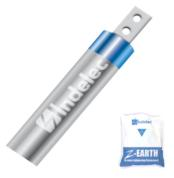
Hot Dip Galvanized with 80-100 micron, corrosion protection, designed for fast fault current dissipation with dual pipe, inner space filled with high conductive material. IS-marked branded mild steel pipe. Electrode systems duly tested and approved by CPRI.
